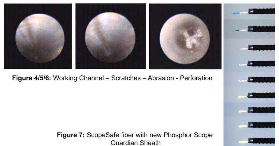
Figure 4/5/6: Working Channel – Scratches – Abrasion - Perforation
