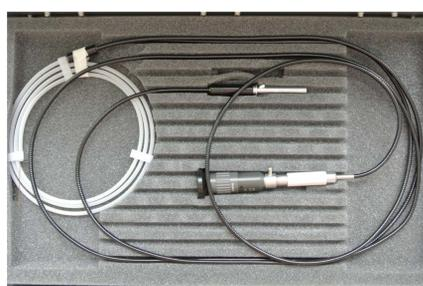
Figure 4: 2.4 Fr Flexible Fiberscope
